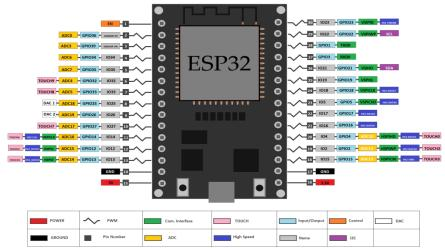
Fig. 4.ESP32 Pinout diagram (30 pin Devkit Development Board)
