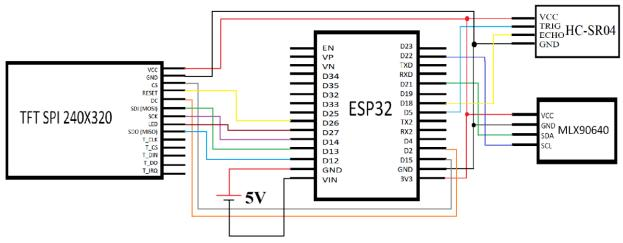
Fig. 5. Circuit Diagram of Thermal camera with distance project
