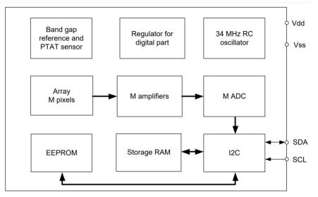
Fig. 2Block diagram is MLX90640
